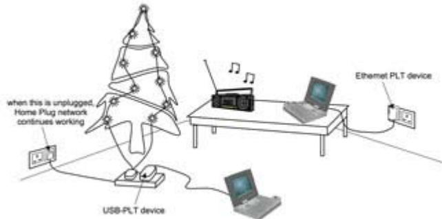
Fig. 6. Arrangement by which a home-networking PLT system can be shown to operate as a wireless network. When the mains extension cable is unplugged from the wall the PLT network continues to operate, despite there being no (wired) connection any more. The broadcast receiver suffers interference when the PLT system is operating, whether 'wired' or 'wireless'.
