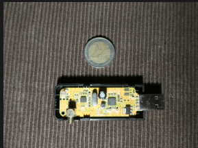
DVB-T USB dongle using the RTL 2832U controller and R820T tuner chip
