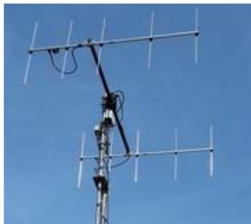
$500W + 16dBd = 57dBm + 16dBd = 73dBm$  ERP (20kW)
