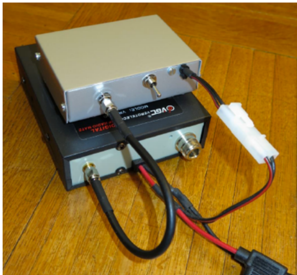
With RF DMR amplifier VR-P25D 20W (Vero-Telecom)
