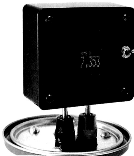
Figure 1 — The RF power display mounts atop the can using banana plugs.
