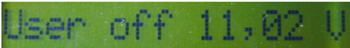
With the button „+“ and „-“, you can define the voltage when the charge regulator should switch off the consumer. Please note that this must not be higher than 10 Amp.
