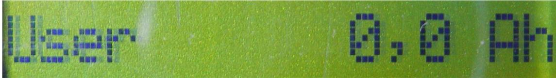
You can also connect a consumer to the screw terminals of the load output and define when the consumer should be switched on and off. The consumer is called user in the picture above. This shows you how many amphours the user has taken.
