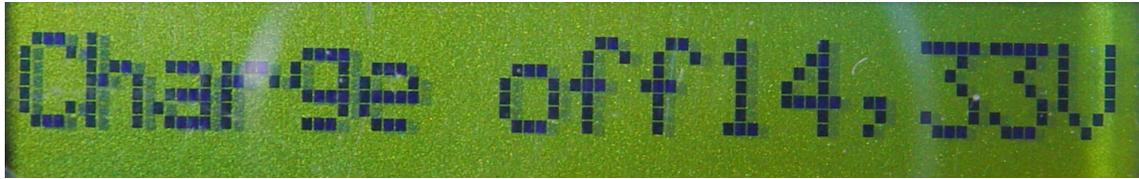
In the display mode shown above „**charge off**“ you can set the max. possible voltage of your battery with the buttons “+” and “-“ . Please note the instructions of the manufacturer of the batteries. The maximum possible voltage is dependent on the system voltage (12/24V) and the type of battery (acid, Gel or AGM)
