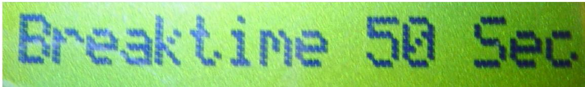
With this setting you can programme the period of time that you want to stop the Silentwind. The longer you programme the time, the longer the first break intervals will take. This procedure will heat up the inbuilt brake resistores resulting in a permanent brake mode until the vent has cooled down. Therefore this time should not be programmed below 50sec.
