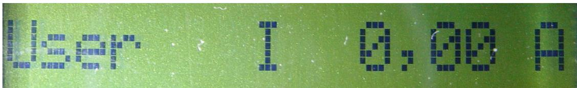
This setting shows how much amps the consumer that is connected to the load output is using.
