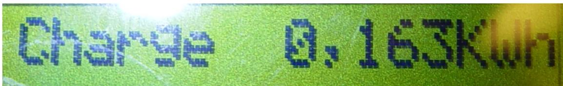
**Charge** shows you the amount of kWh have been loaded into the battery. This parameter is updated every 10 seconds.
