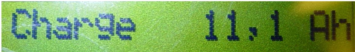
**Charge** shows how many ampere-hours (Ah) have been charged into your battery. This is updated every 10 seconds.
