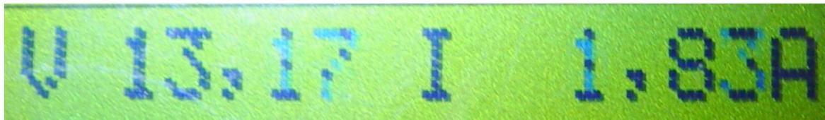
In the display mode you can see above the battery voltage and the charge current. The total current (wind and solar) is shown.
