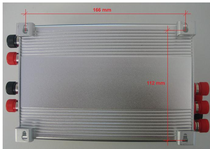
As you can see from picture 2 there are 4 mounting holes on the back of the charge controller. Use filister head screws with appropriate (suitable) diameter and screw them into the mounting surface according to the measurements shown in the picture above. Don't screw them completely into the mounting surface. Place the mounting holes over the screws and slide the charge controller into the 4 slurry wall trenches. Screws are not included in delivery.
