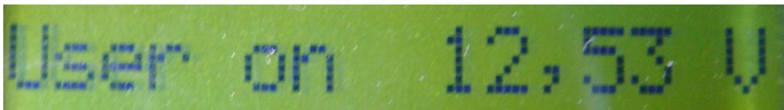
User on defines the voltage when the consumer can be switched on again. As the voltage of the battery increases when switching off the consumer this will steadily switch on and off the load output if this value is not high enough. This function can also be used with smaller batteries.. So that the charge voltage is not detected too fast, you can connect a consumer additionally. This avoids that the brake will be activated too early.
