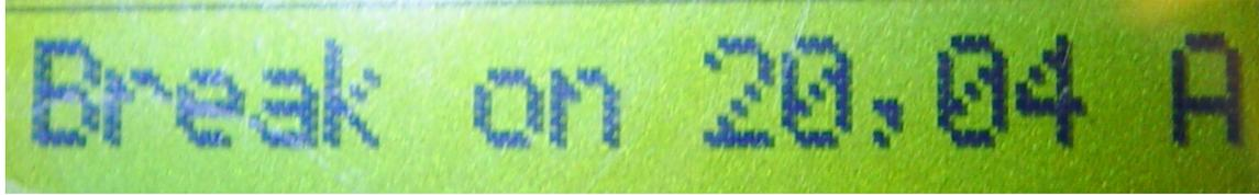
With +/- you can set the current when you want to stop the Silentwind Generator. This prevents overheating, especially with big battery banks and high loading currents. This function can also be used to reduce the RPM of the Silentwind Generator.
