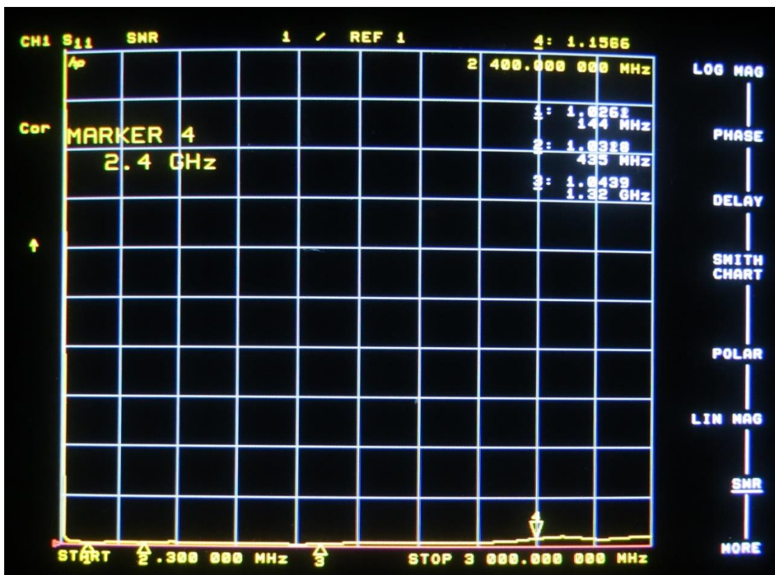
S11 SWR 300 kHz – 3 GHz
