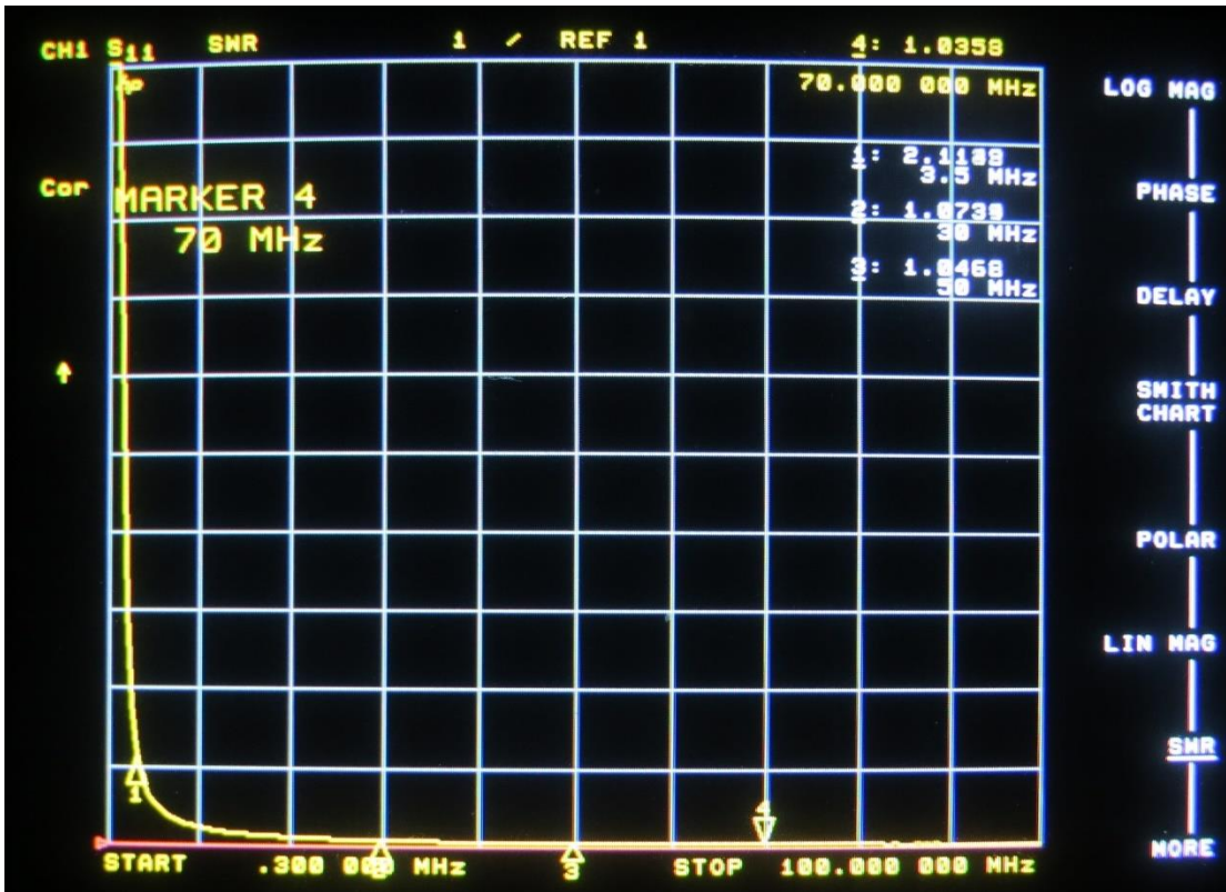
S11 SWR 300 kHz – 100 MHz
