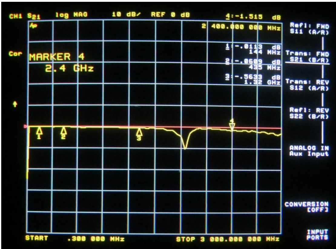
S21 LogMag 300 kHz – 3 GHz
