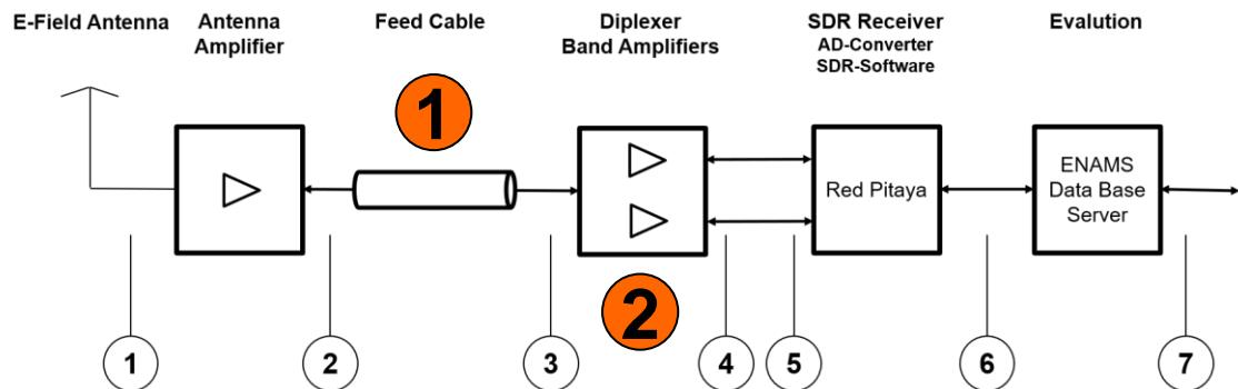
$$P_{50\Omega} = C_{SDR}(E_{Ant}, f, T, M) \cdot V_{Filter}(E_{Ant}, f, T, M) \cdot D_{Kabel}(E_{Ant}, f, T, M) \cdot k_{Ant}(E_{Ant}, f, T, M) \cdot E_{Ant}(f)$$
