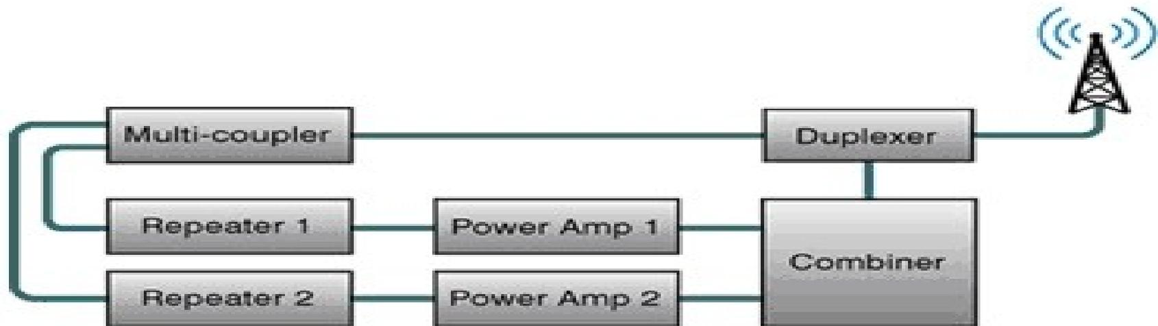
Repeater Equipment for Two Channel FDMA
