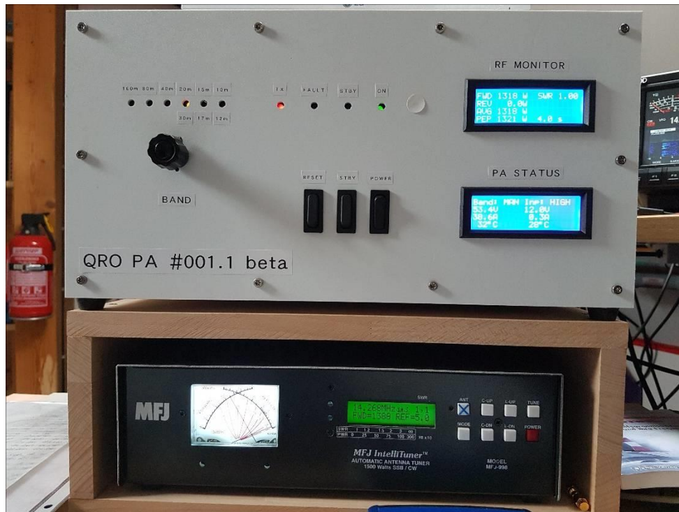
BETA, thermal test 1.3kW+ continuous
