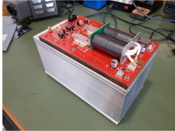
RF PA using 2x LDMOS is waiting
