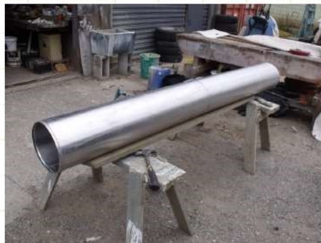
Overlapped and screwed together with self tapping screws
