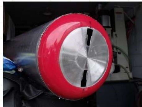
Back home.....slots in base to insert coupling loops and connectors
