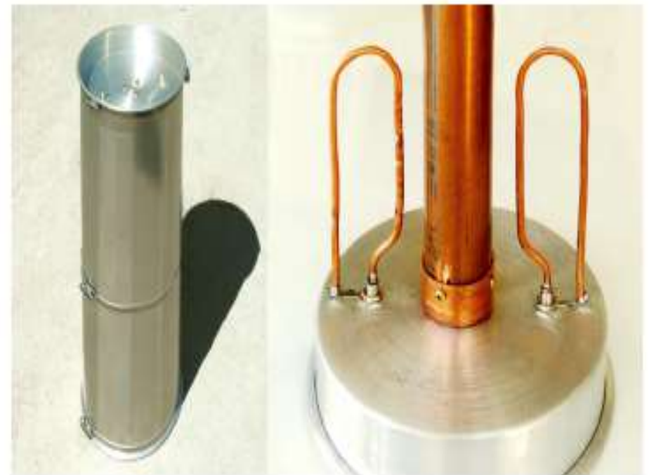
Figure 2-2: Example 2M cavity and loop detail
