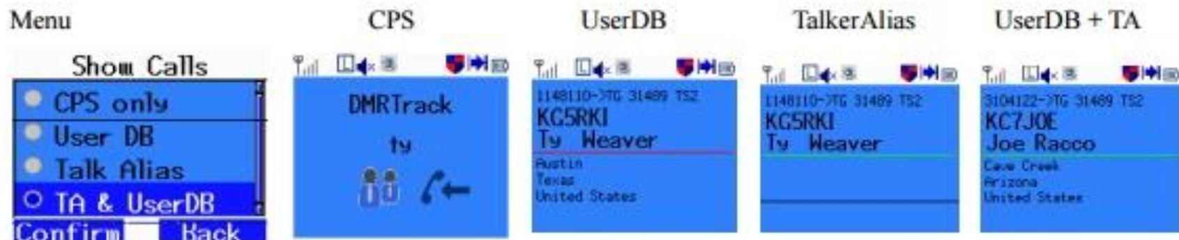
This will change the receive screen that is shown while receiving a transmission. Normally only the talkgroup name and DMR ID / contact name is shown. By changing these options, you enable the use of a user database which contains all of the data for the DMR Ids in the system. The talker alias option will display the TA data if available.
