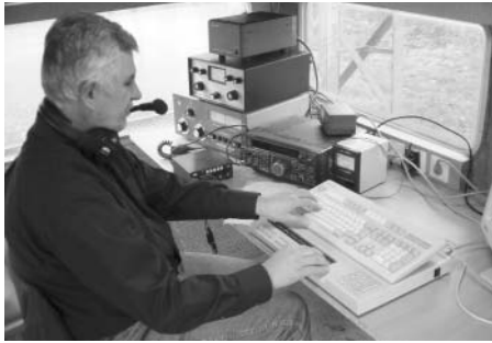
DL2VB, at the controls of DL0GL. Marvin is blind and uses a Braille display which allows him to read text on the screen. You can see this below the keyboard. Using the popular TR software by N6TR, he is able to log QSOs and QTCs without help, up to four QSOs per minute.
