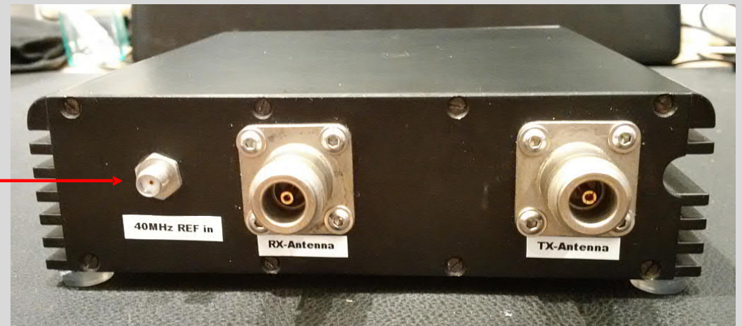
ADALM Pluto in shielded encasing with external 40 MHz reference input
